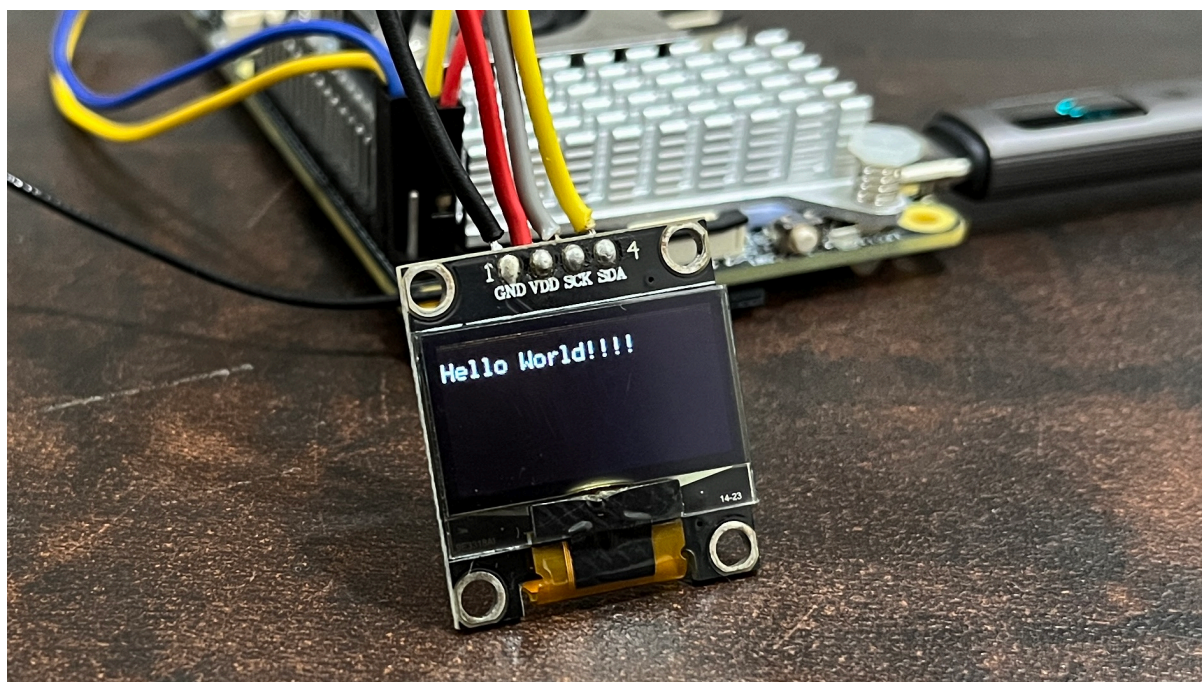
Fig. 5.21: Hello World!!!! on 128x64 OLED
