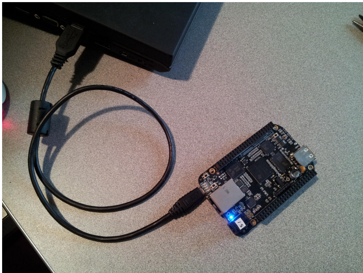
Fig. 15.1: Plugging BeagleBone Black into a USB port
