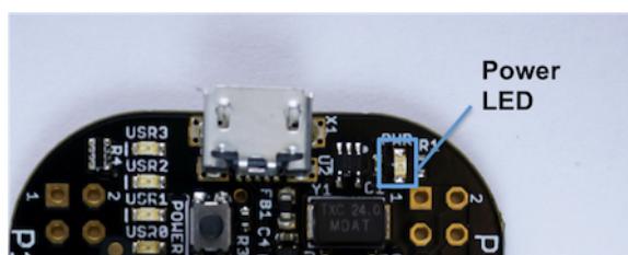
Fig. 11.14: Board Power LED
